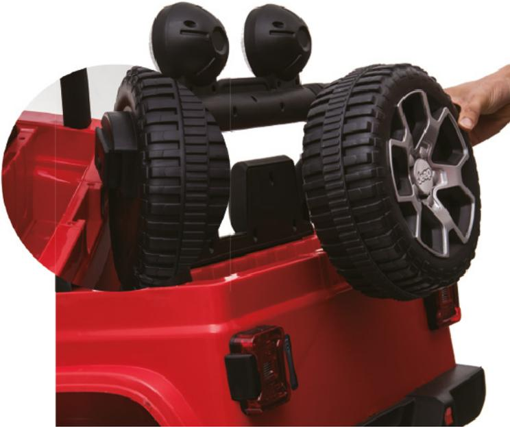
Install as shown in the photo, locating the spare wheel in the rear slot and fitting it correctly.
