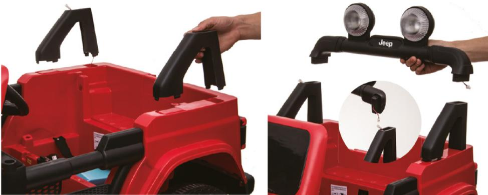
First fit the brackets for the lights by pressing them down at the rear of the car. Subsequently, fit the lights to the brackets in the same way.
