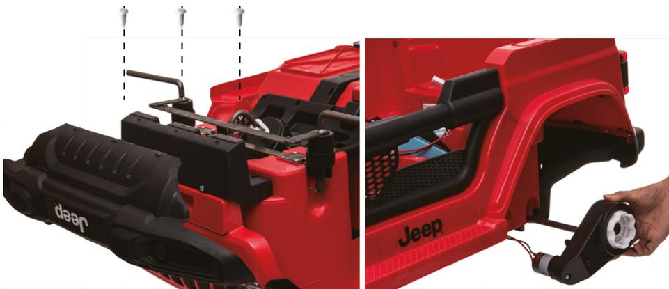
Insert the motors into the axles and insert the screws into the holes in the body. Reconnect the power cables.
