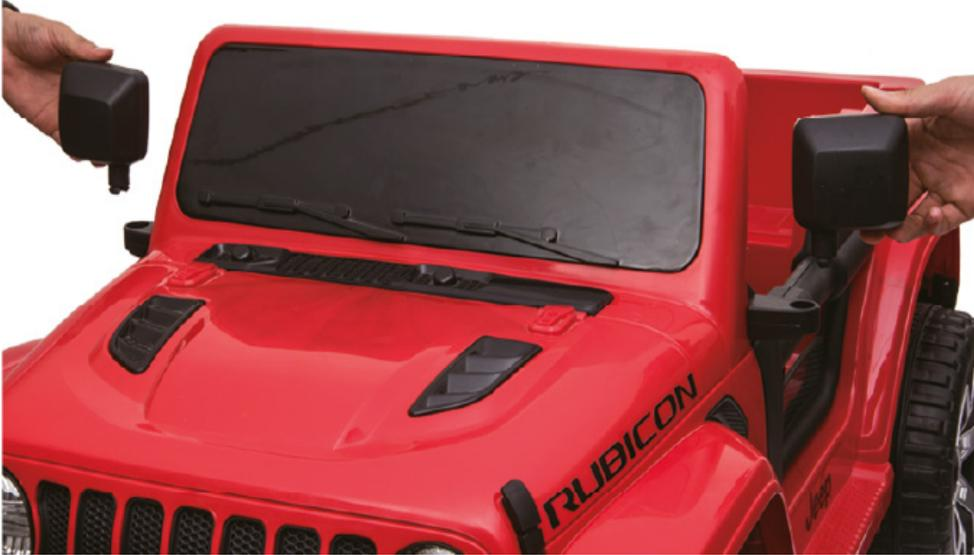
Position the rear-view mirrors by pressing down until it locks into place.
